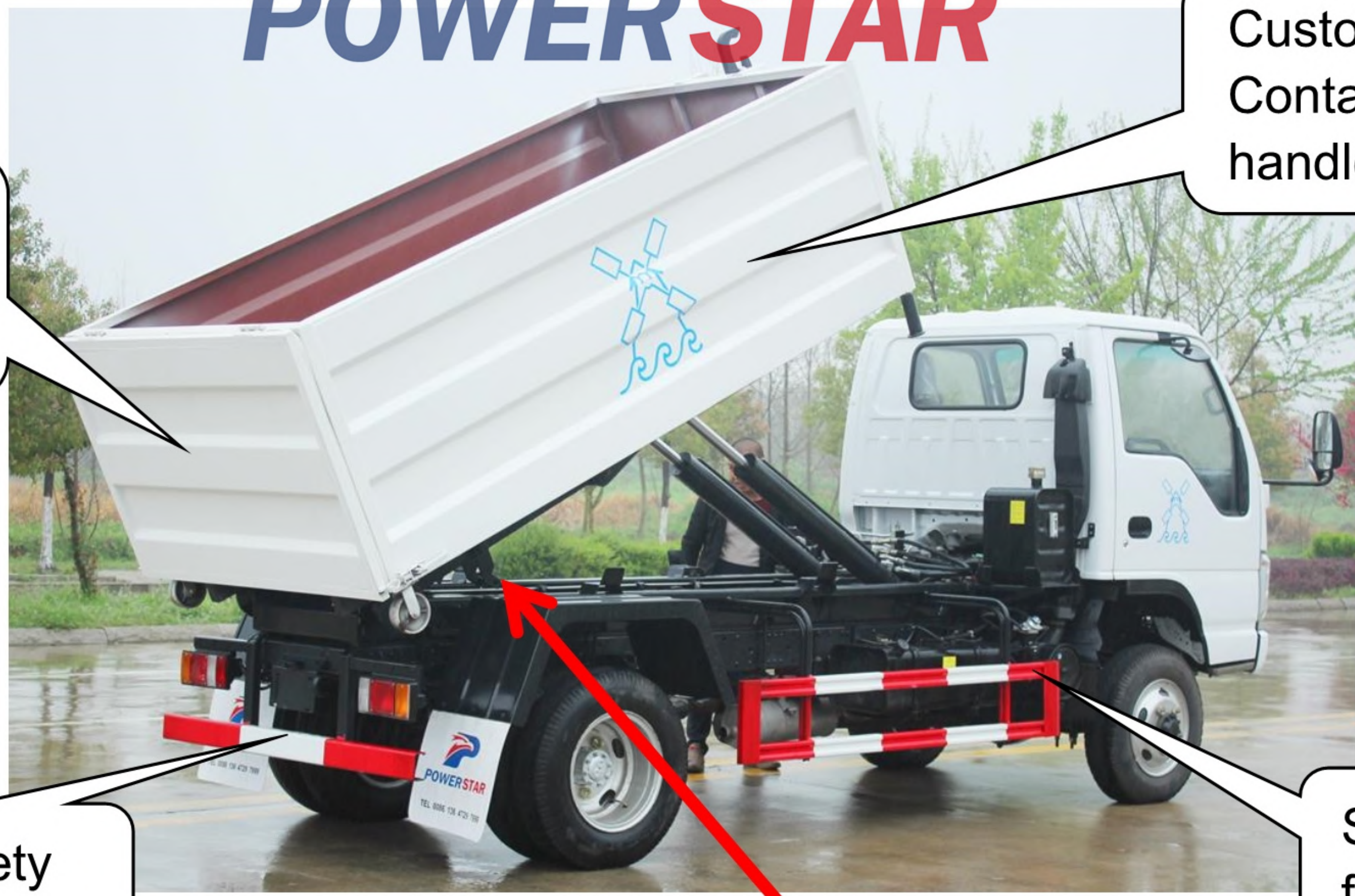
Rear View: Customized garbage containers with rear door & safety fence.
